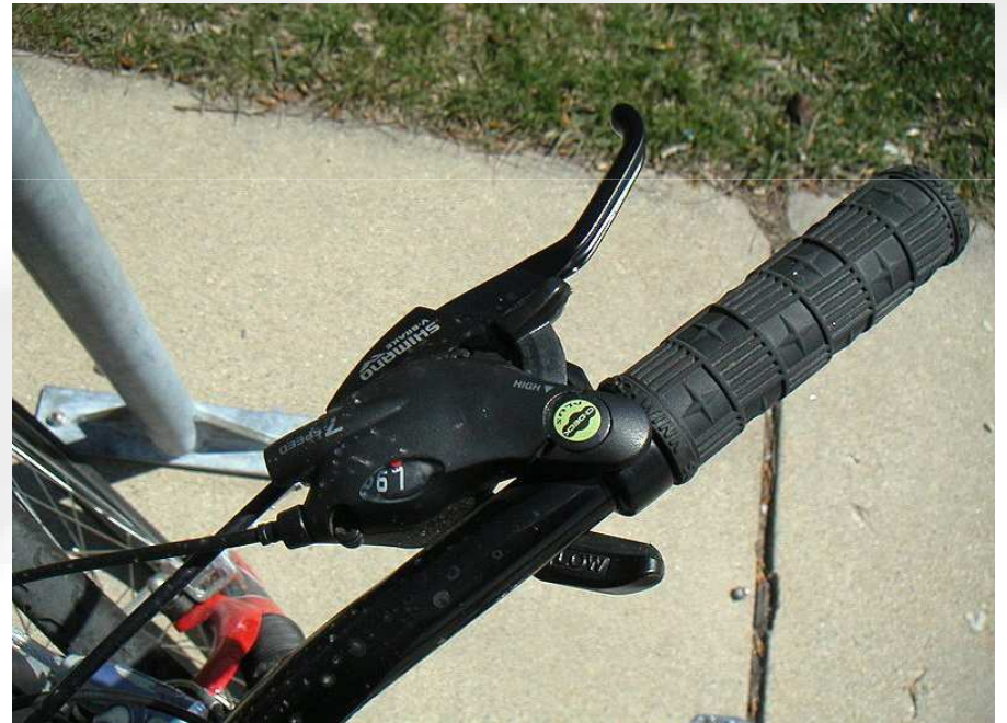
Index shifter with integrated brake lever
